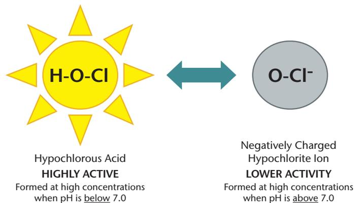
**Figure 2.** Transition of hypochlorous acid to hypochlorite ion in different pH conditions.
